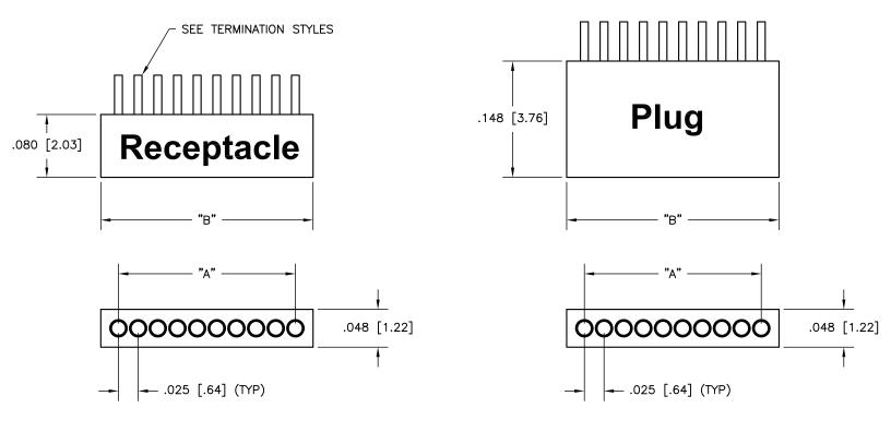
A = (NO. OF POSITIONS -1) X .025 [.64] 1ST TO LAST CONTACT B = A + .050 [1.27] = OVERALL
