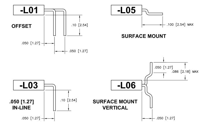
RECEPTACLE (SOCKET) TERMINATIONS ARE SELF-LEAD (ONE PIECE) .014 [.35] DIAMETER
