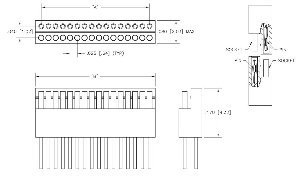
A = (NO. OF POSITIONS IN SINGLE ROW -1) X .025 [.64] 1ST TO LAST CONTACT
